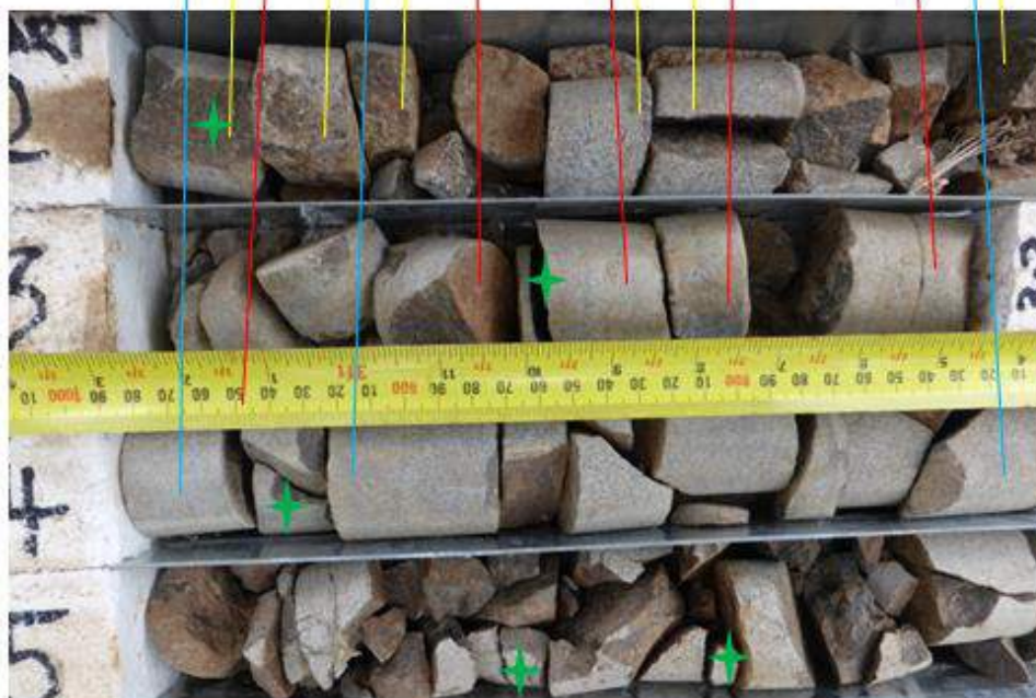
Figure 5 Comparison of core from MVDDH6 2006 and 2015 showing little change. Coloured lines link the identical pieces of core + indicates new breaks in core since 2006
